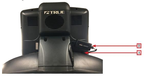
Route the longer cable with the infrared (IR) blaster downward and inside of the pedestal upright. Note: The red line in the picture is the suggested cable routing.
